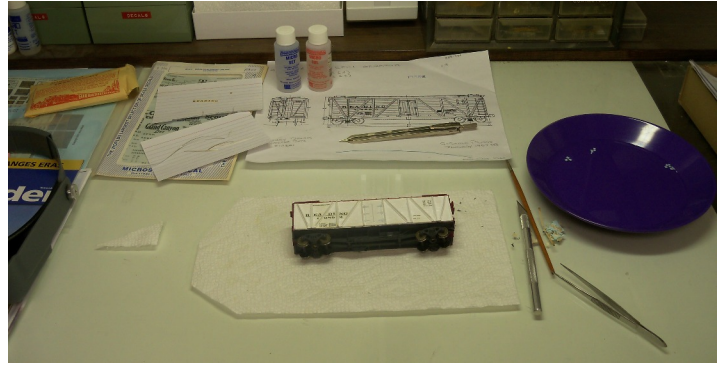
Decaling is done on a glass top desk with a water bowl, tweezers, hobby knife with #11 blade, dividers, setting solutions and a small paint brush.
