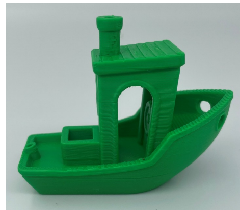
Figure 6: 'Benchy' model for benchmarking 3D printer performance, printed out of the box
