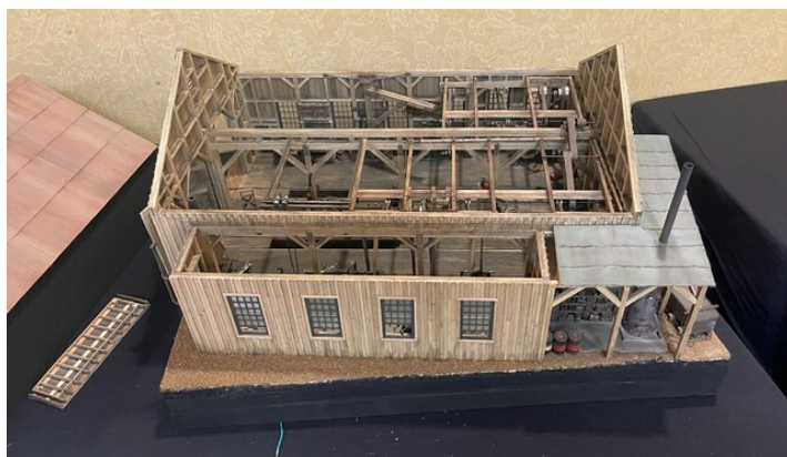
Operating model of a machine shop with lights and overhead belt and pulley power.
