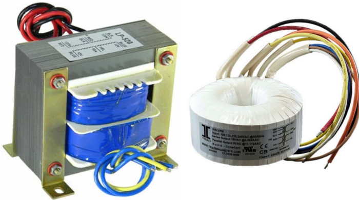
Figure 4: Hammond Manufacturing 165P30 150VA 30V CT 5A Transformer, former Laminated (Mouser #546-165P30 or Digikey #HM561-ND) Figure 5: Triad Magnetics VPM30-3330 100VA 30V CT 6.66A Parallel, former Laminated (Mouser #546-3330 or Digikey #237-2040-ND)
