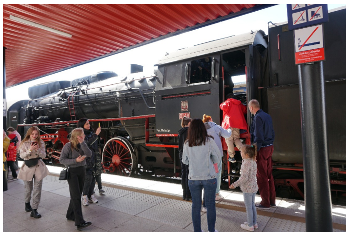
Youngsters get a tour of the locomotive cab. The OL49-69 is a standard Polish 2-6-2 built in 1953/1954 and designed to pull six loaded passenger cars at 55mph.
