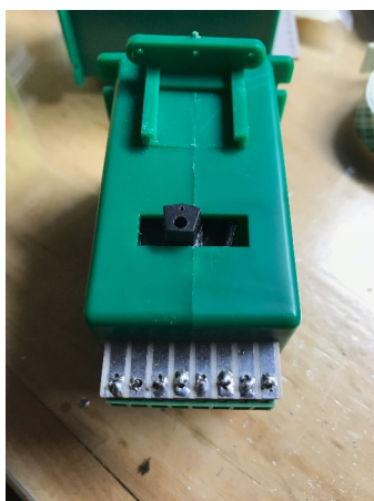
I soldered the pins to make connectivity. This picture made me realize I needed to redo a couple of them.
