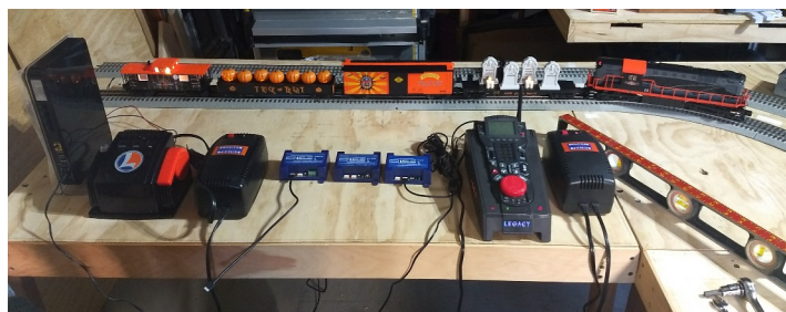
Command Console mockup - WiFi router, GW-180 and PowerHouse 180, remote switch controllers, Legacy base, and second PowerHouse 180.
