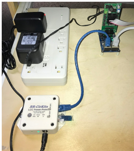
XO Tower consists of an LCC Power Point that provides power to the network, and a Tower LCC board that holds the SMD-8 daughter boards that connect to the turnouts. The grey cable goes to the laptop that connects with an LCC Buffer USB
