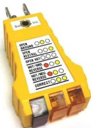
Figure 3 Ground Plug with Circuit Check
